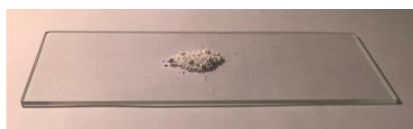
Fig. (1) The silicon nitride nanopowder extracted from thin film samples prepared in this work
