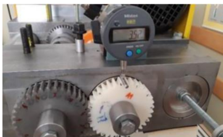
Fig. (3) Measurement setup of the gearbox parts
