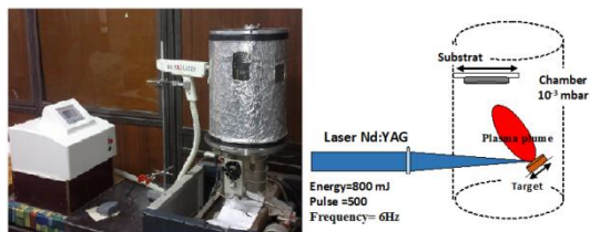
Fig. (1) The experimental setup of PLD used in this work
